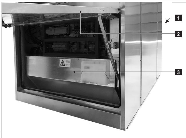
Fig. 13: The fan protecting plate is temporarily attached with 4 screws during delivery.
