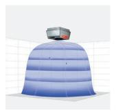
**Cooling operation:** The inflowing air is colder than the room air and sinks. To avoid draughts, it is injected horizontally.
