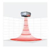
Heating operation: The supply air is warmer and thus lighter than the room air. The vertical inflow of air ensures that the heat reaches the areas where it is needed.
